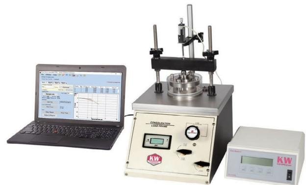
Figure 2: Pneumatic Consolidation frame with 1in Displacement Transducer and Two-Channel Data Readout Box
