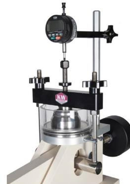
Figure 1: Dead-Weight Consolidation Frame with Digital Dial Indicator
