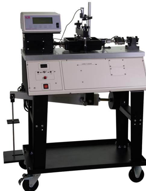
Digital Dead-Weight Direct Shear Machine (shown with Shear Box sold separately)
