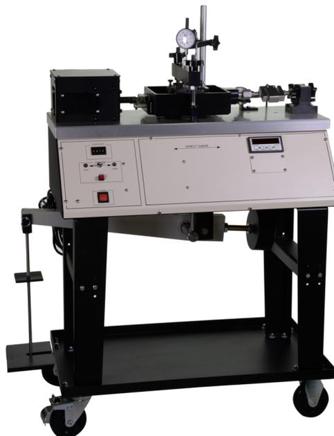
Standard Dead-Weight Direct Shear Machine (shown with Shear Box sold separately)
