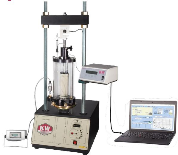
Figure 1: Typical triaxial test setup
